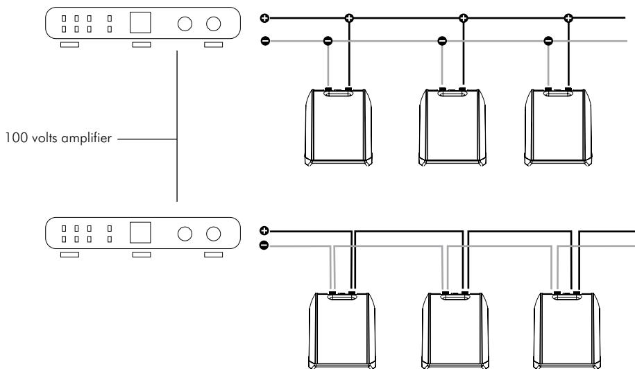
The electrical connections on "4 Ω" mode
