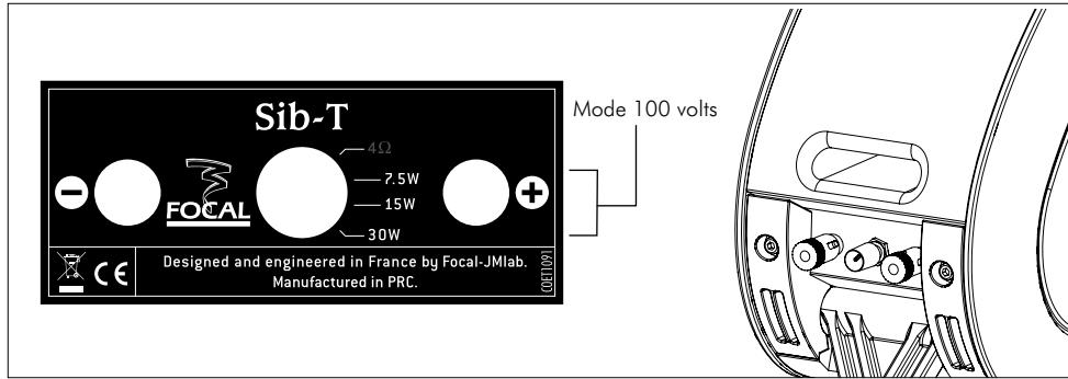
**Warning!** Before turning the system on, make sure that your amplifier is on 100 V mode.
