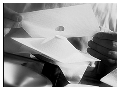
The hand-made manufacturing of the "W" cone. Our industrial process is patented.
