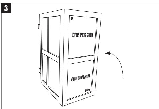
3 - Put up the box of Maestro body, being careful about the up and down sides.
