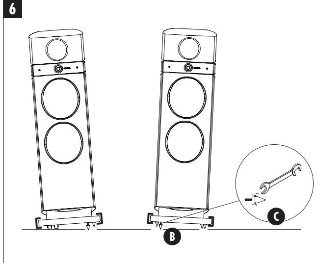
**6 - Once the position is chosen, topple over the loudspeaker on its side (with the protection foams in place) to insert the spikes. You can use protection cups to protect the floor. 2 people required.**
