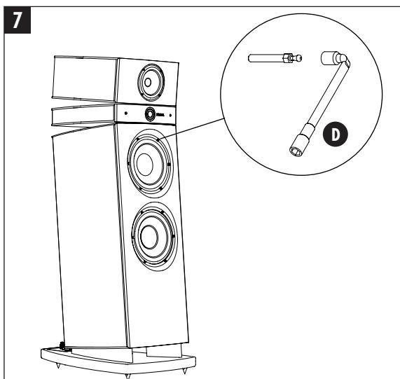
**7 - For safety reasons, screw all the speaker screws (woofer and midrange) that could have been unscrewed during transport. Use the supplied tube wrench.**
