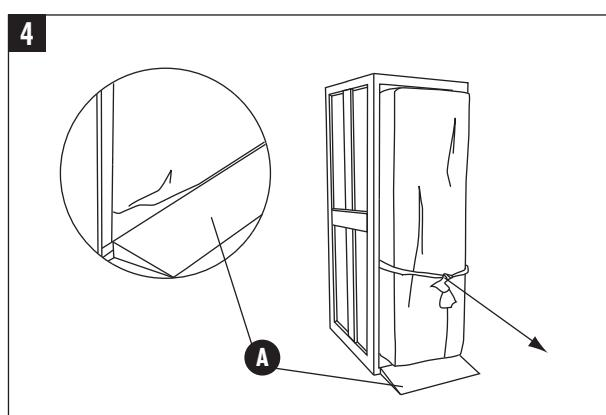
4 - Install the ramp as indicated. Carefully pull out the loudspeaker thanks to the girth.
