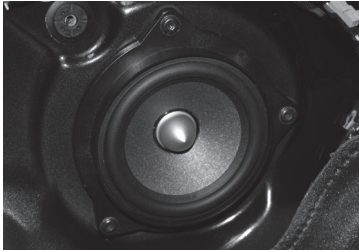
7. IFBMW-S assembled in the door.
