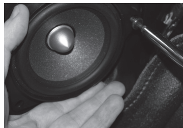
6. Assembly of the IFBMW-S speaker.
