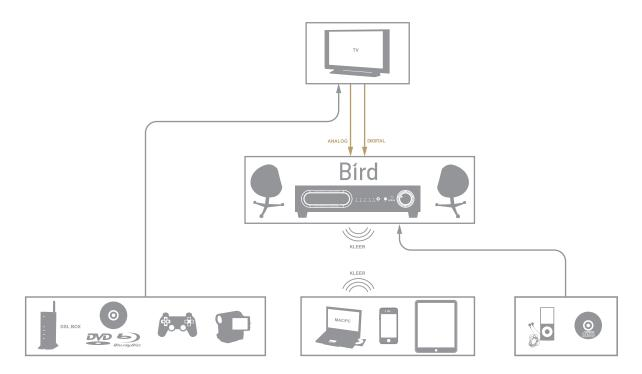
The Little 2.1 Bird system needs no configuration or set-up as it will play right out of the box (cable and mounting accessories supplied). The audio/video sources can be connected to the TV set and the sound is then redirected towards the Power Bird. In this installation, you will hear the signal that corresponds to the image on the screen. Audio sources can also be directly connected to the Power Bird and there is no need to consult the screen.
