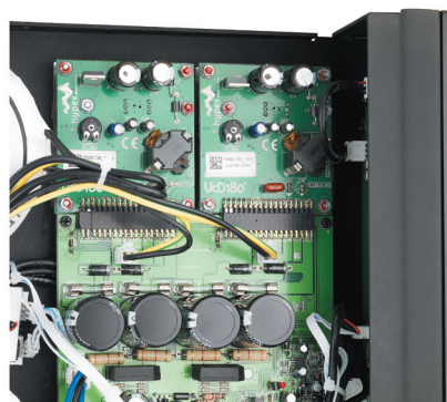
- Stereo power component class D Hypex
