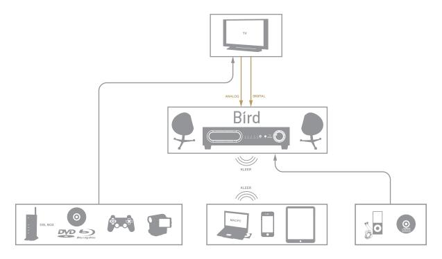
The 2.1 Little Bird system needs no configuration or set-up as it will play right out of the box (cable and mounting accessories supplied). The audio/video sources can be connected to the TV set and the sound is then redirected towards the Power Bird. In this installation, you will hear the signal that corresponds to the image on the screen. Audio sources can also be directly connected to the Power Bird and there is no need to consult the screen.
