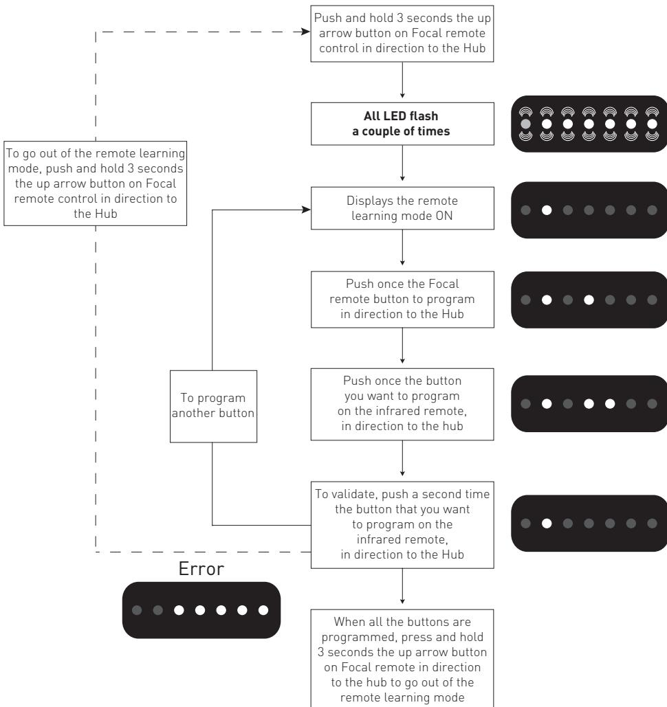
**Note :** To erase programming on the Infrared remote control, press and hold for 10 seconds the up arrow on the remote Focal. If no key is pressed for 1 minute then programming mode will become inactive.
