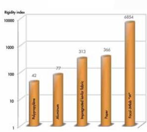
With equal cone mass and diameter, the rigidity and flexibility index of the "W" sandwich outclasses the most employed materials.
