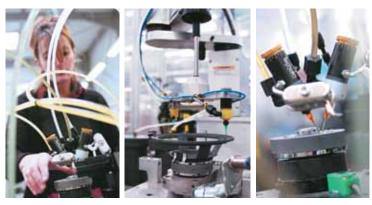
> Our assisted build woofer production line allows us to retain the values of a traditional hand built driver.
