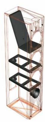
> The ever-present attention to detail is the trademark of a high-end Focal product. Aside from the MDF construction up to 25mm in thickness, multiple internal reinforcements, which also integrate the routing of the cables, the non-parallel structure of the inside walls, the quality of finishing where each detail is maintained from the design stage... all this makes for cabinets that are truly unique in this price category.
