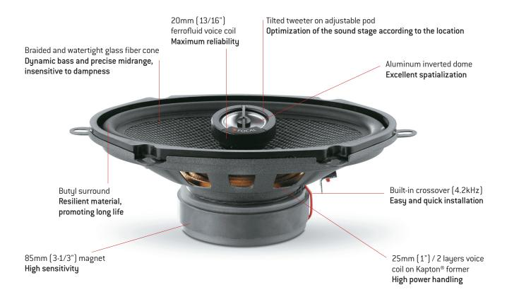
130 x 180mm (5 x 7") woofer 25mm (1") voice coil 85mm (3-1/3") magnet Aluminum inverted dome tweeter Built-in crossover (4.2kHz) 6dB/octave Max. power: 120W - Nom. power: 60W Sensitivity (2.8V/1m): 91dB Frequency response: 65Hz – 20kHz
