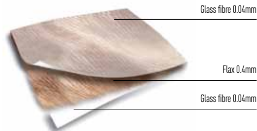
FLAX sandwich cone 6 1/2" (165mm) woofer cone conception
